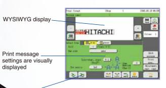
Various parameters, such as the line configuration and font size, can be easily set on a single screen.
